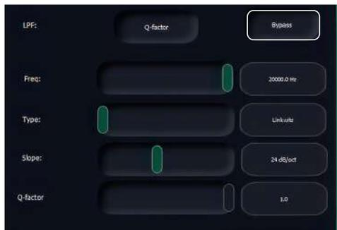
To temporarily disable the selected filter without resetting its settings, click the BYPASS button next to the filter name
